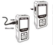
Open the cap and insert the USB recharging cable with Mirco-USB Port
