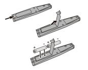
Change batteries when battery symbol is empty.
